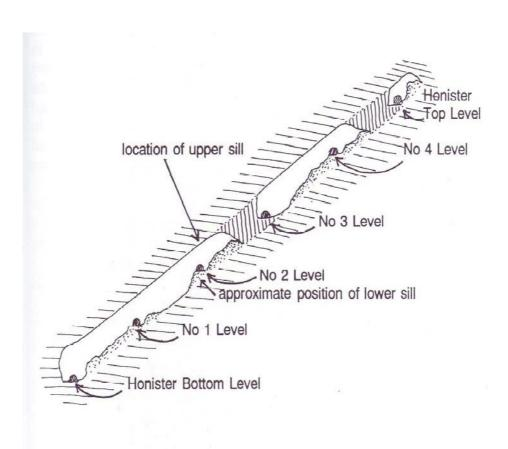
A cross sectional diagram of part of the worked out area of the Honister Band. The diagram shows that Honister Bottom Level, No 1 and 2 Levels have all connected although they were once separate chambers. The well-defined upper sill is clearly evident but the position of the lower sill is almost completely obscured by debris. The No 3 and 4 Levels are also connected.
